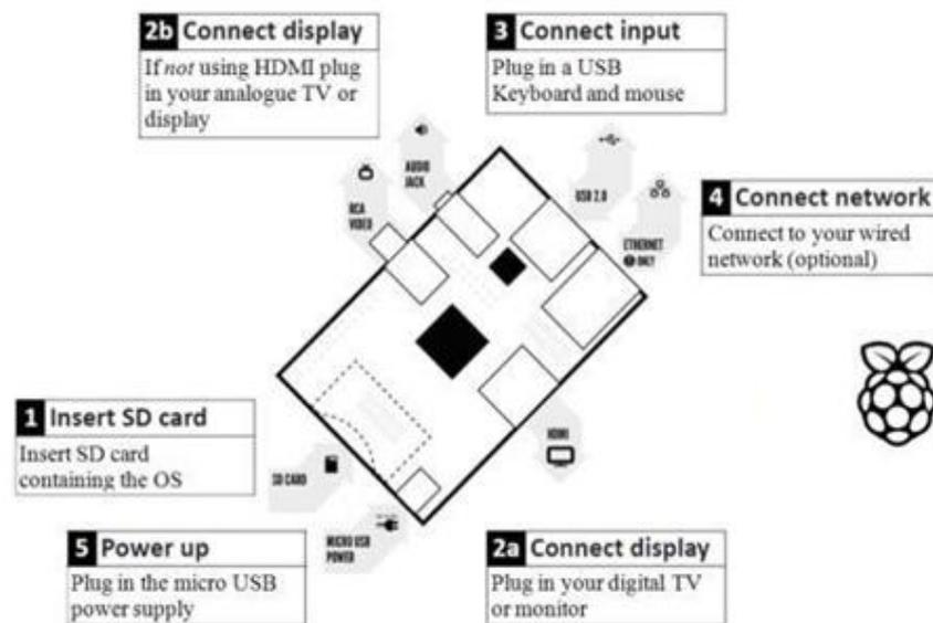
**Fig 2.** Description of raspberry Pi Board.
