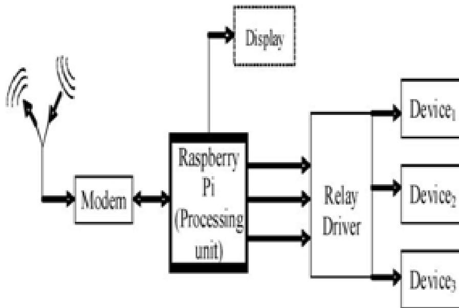
Fig 3. Layout of the basic home automation system configuration.
